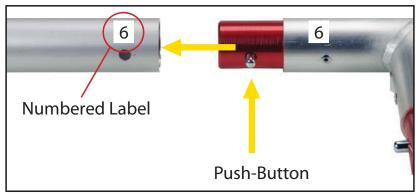
Connections are made by holding the button down and sliding the red tube into opposing tube until the connection is made. To disassemble push button and pull or twist extrusions apart.
